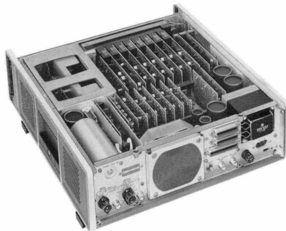
Fig. 12. Circuitry in counters is built up on removable computer-type circuit boards to achieve compact overall size and high accessibility.
